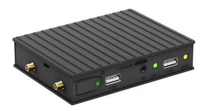
IOT-GATE-iMX8PLUS is a powerful Industrial IoT Gateway PC based on the iMX8M Plus processor designed for IOT control and monitoring applications.
